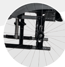
Choice of four centre of gravity settings
